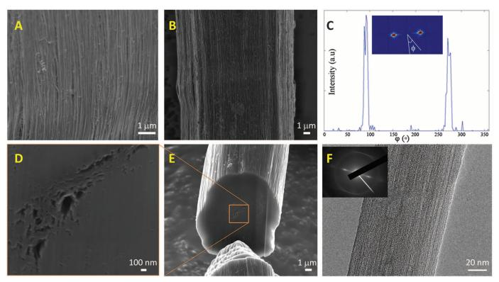
**Fig. 3.** (**A**) High- and (**B**) low-magnification SEM showing the typical morphology of CNT fibers composed of ~100-nm-thick fibrils aligned along the fiber axis. (**C**) Single-fiber x-ray diffraction (inset) and azimuthal scan showing the high fiber alignment. (**D** and **E**) SEM images showing fiber's cross
