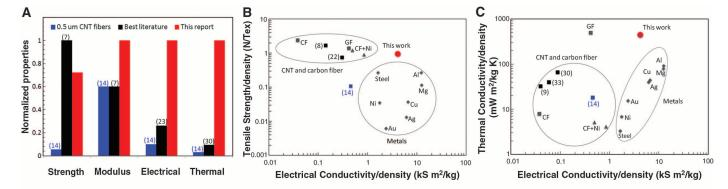
**Fig. 2.** Properties of continuous, neat CNT fibers. Black denotes literature values (7, 8, 9, 22, 23, 30, 33), blue denotes earlier wet-spun 0.5-μm CNT fibers (14), and red denotes fibers in this report. (**A**) Comparison of properties normalized to the highest value. (**B**) Ashby plots of specific tensile strength versus specific electrical conductivity of metals (gray diamonds), pitch (GF) and PAN (CF) carbon
