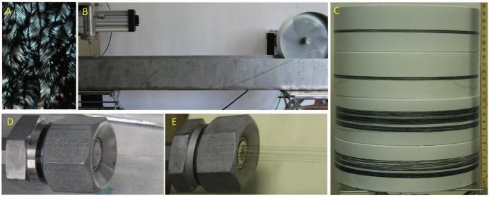
**Fig. 1.** (A) Light micrograph of a birefringent fiber spinning dope (3 wt % CNT in chlorosulfonic acid). (B) Fiber spinning set-up. The fluid is extruded from the spinning chamber (left) through a spinneret immersed in a coagula-
