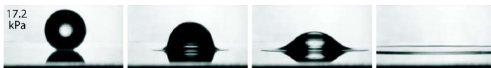
Fig. 7 Sequence of the drop deformation under very low ambient pressure. Photos courtesy of Lei Xu and Sidney Nagel
